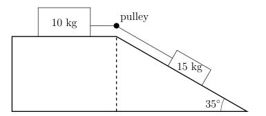
b) Find the acceleration of the system correct to the nearest  $0.01 \text{ ms}^{-2}$ .
