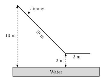
**b)** Show that Jimmy accelerates down the incline plane at  $5.488 \text{ m/s}^2$ .
